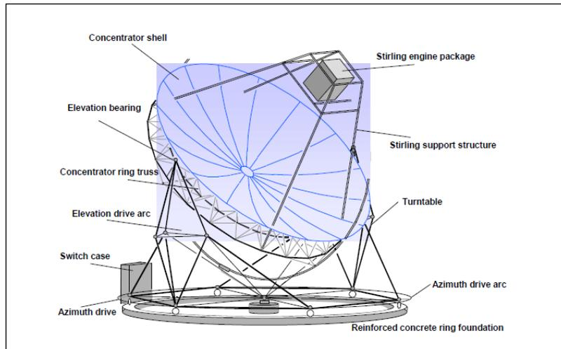
**Figure 3: Dish Stirling system**
