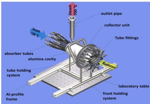
**Figure 6:** Tubular solar receiver
