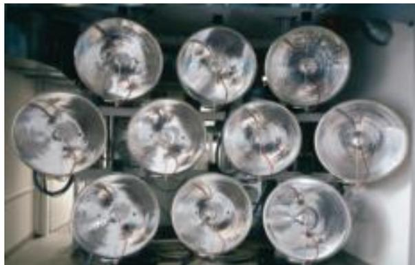
**Figure 5:** Xenon high flux solar simulator
