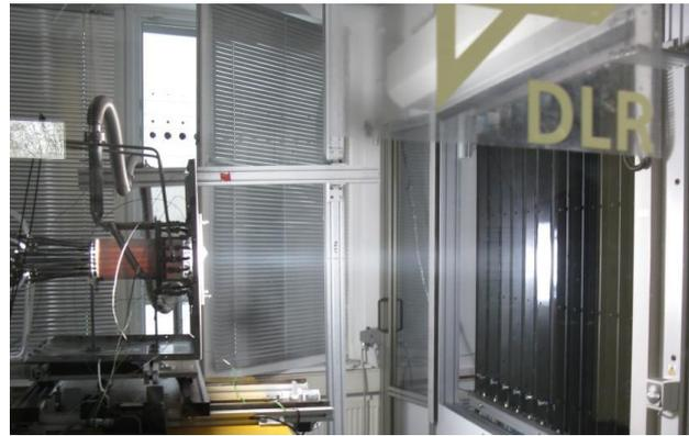
**Figure 7:** Tubular solar receiver tested in the DLR's solar furnace
