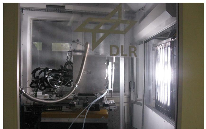
Fig. 3 Irradiated solar receiver in DLR's high flux simulator
