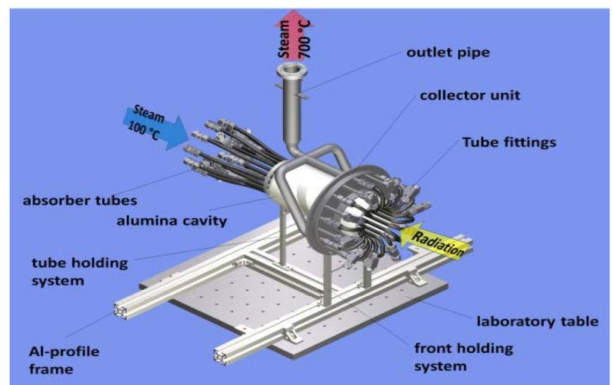
Fig. 2 CAD model of solar receiver
